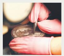
2 Engravers help to touch up the design after it is transferred from the mould to the working die.
