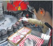
Meanwhile, the blank coins, which are either bought from overseas or produced by the mint itself, are being buffed to a shine with a machine.
