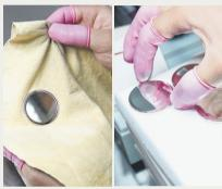
4 The blank coin is checked and cleaned a final time by hand before the design is pressed onto the coin.
