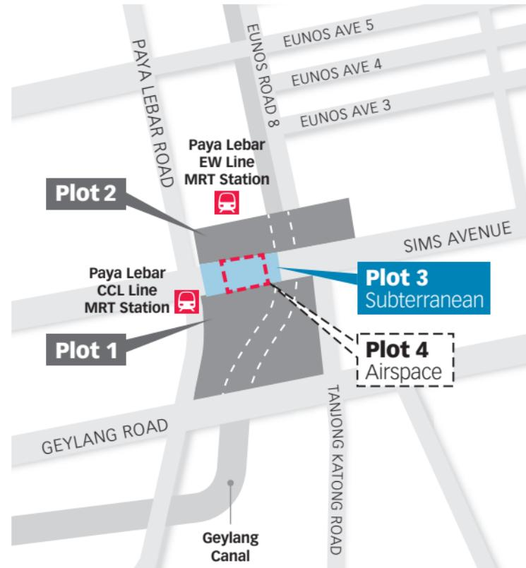
Plot 3 – Subterranean space for an underground vehicular and pedestrian connection between Plots 1 & 2
